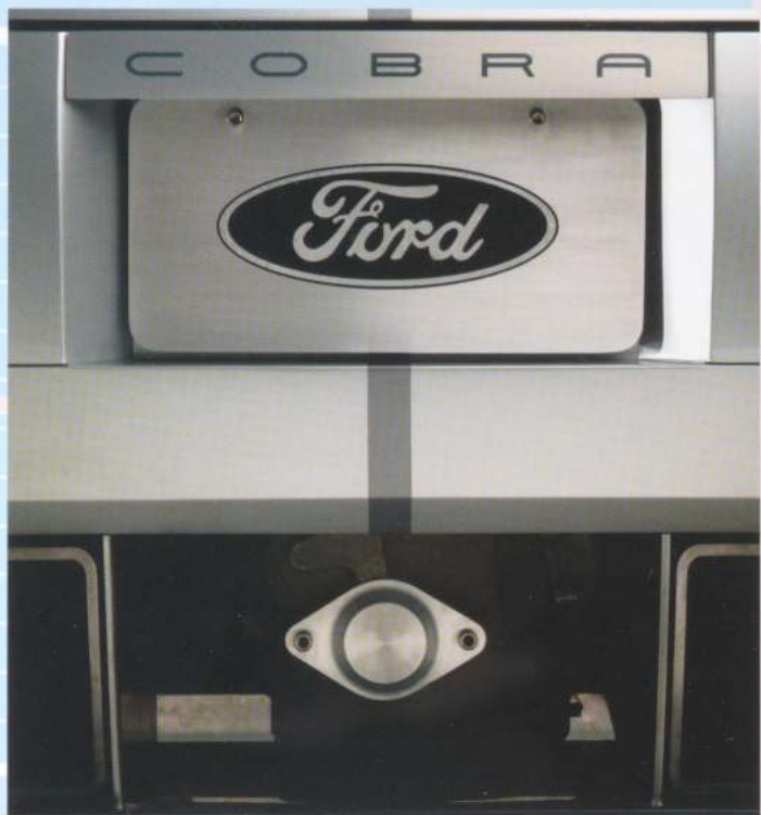
The machined rear face of the six-speed transaxle becomes a design element, flanked by two huge exhaust openings.
