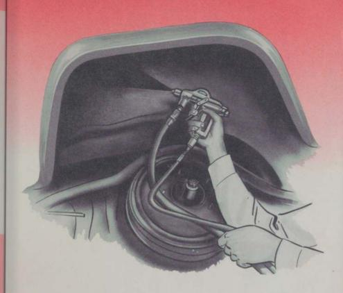
Get increased riding comfort from your car and preserve its trade-in value with an application of FoMoCo Undercoating. Undercoating protects the under surfaces of your car against water, salt spray, road chemicals and flying stones—keeps body bolts tight—seals metal-to-metal seams. It forms a resilient cushion that deadens sound, and acts as an insulator against heat and cold. You may also notice that it gives a heavier, more luxurious "feel" to the car.
