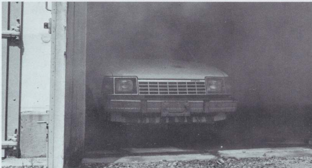
To test toughness against corrosion, prototype World Cars covered with salt spray and road dirt were parked in a "steam bath" chamber at 120 degrees and 95% humidity for 22-hour periods.
