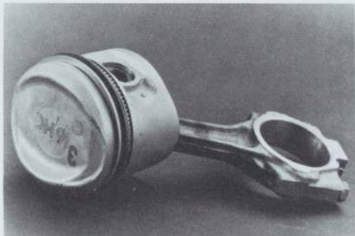
Close-up of engine block and crankshaft (top). Each piston's head is contoured so it forces the fuel/air mixture toward the center of the combustion chamber, boosting engine efficiency.
