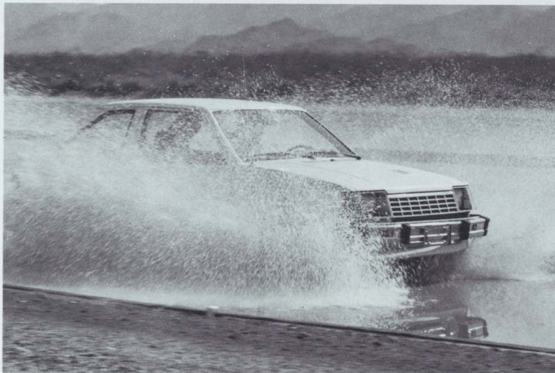
A Ford Escort plows through a pool of brine to test its salt resistance at the Arizona Proving Ground.
