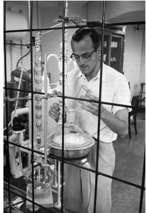
In his sleuthing for trace amounts of lead, Caltech geochemist Clair Patterson redistills a reagent in this 1957 photograph. He didn't trust the purity of commercial chemicals.
